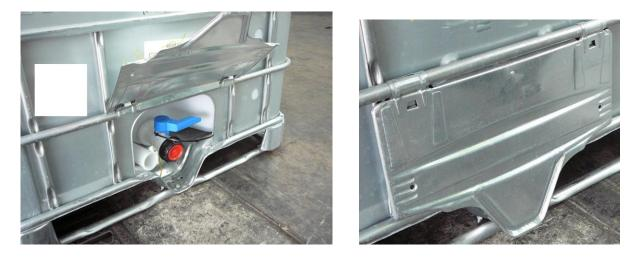
40. Metal IBCs may also fail hydraulically or by ullage space explosion. Consideration could be given to the fitment, whilst in storage, of pressure relief valves to reduce the risk of catastrophic failure in the event of fire. If a third party under contract supplies the IBC, this should be done with their permission and restored to UN specification prior to transport.
